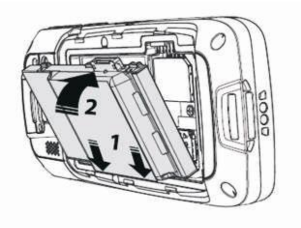
Figure 1-22: Inserting the 4,410 mAh Battery
